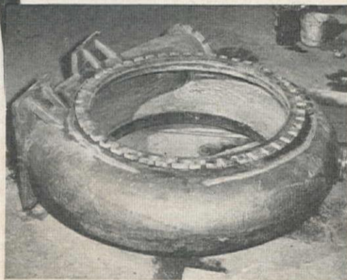
DREDGE PUMP CASING —A typical application of Stooddy Self-Hardening 21. A 1/4" single pass layer is applied manually to the new casing. May be reapplied as needed.
