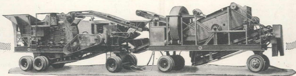
Two-Unit Portable Crushing and Screening Plant
