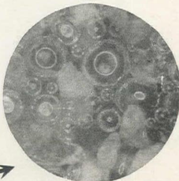
Photomicrograph of sand paste mixed with Darex AEA showing entrained air bubbles separating particles of sand.
