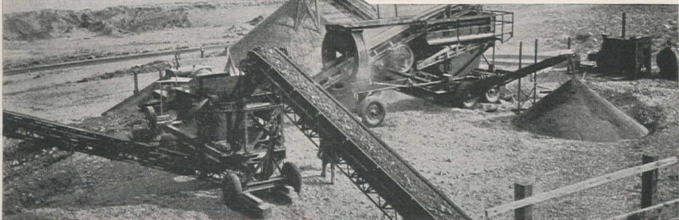
Two-Unit Portable Crushing and Screening Plant.
