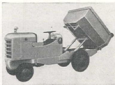
Features claimed: The four-wheeled, pneumatic-tired unit is powered by a gasoline engine and has a hydraulically-dumped body. It is built low and compact with a short wheel base and rear wheel steer so it can operate in congested low head-room areas and through narrow doorways. Overall height is 5 ft., 8 in. Hydraulic brakes plus full visibility in every direction allow high speed travel with complete safety.
