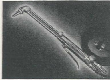
rigidity and heat resistance. The stainless steel lever and ribbed handle are designed to afford maximum ease of operation. A remote control cut-off automatically coordinates the flux feed with the cutting oxygen, eliminating separate flux control. It uses standard cutting tips and has a monel metal head for durability. The new torch is available in 21- or 36-in. lengths, both having a 90 deg. torch head.
