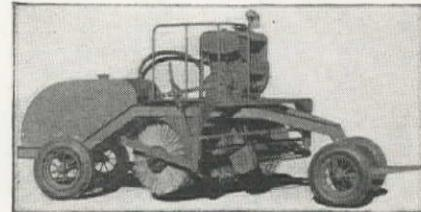
**Features claimed:** The unit will pressure flush and sprinkle streets, clean sewers, sweep wet or dry, spray trees and shrubs and fight fires. A full width water blanket spray in front of the 7-ft. brush prevents dust clouds ordinarily associated with dry sweeping. The brush life is lengthened by constant wetting through auxiliary piping.
