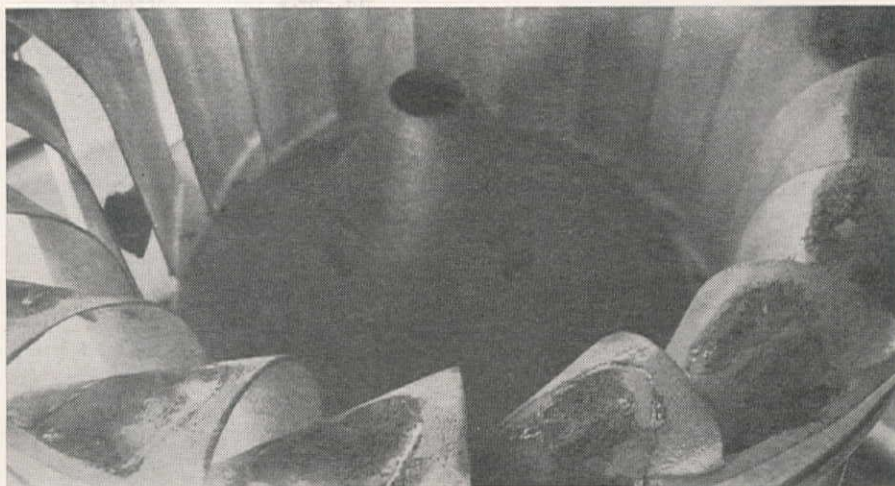
LARGE HOLES in the bucket and weakened areas in vane and shroud of the turbines were caused by cavitation effect in the hydraulic stream. Before and after views, above and below, show how original shape and thickness were restored. The 15,000-h.p. Francis type turbines were repaired at one-fifth estimated cost of new runners.
