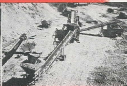
PORTABLE CRUSHING AND SCREENING PLANTS—Range in size from a mounted crusher to the magnificent Two-Unit and Three-Unit Plants. Illustrated is the new "101" with its jaw and roll crushers.
