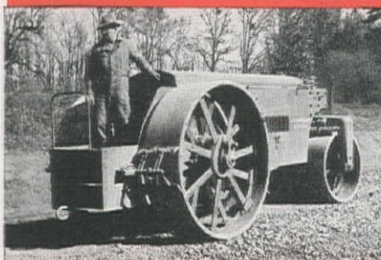
3-WHEELED ROLLERS—Made in sizes ranging from 6 to 12 tons. Gasoline or Diesel engines. Hydraulic power steer. Hydraulic scarifier attachment.
