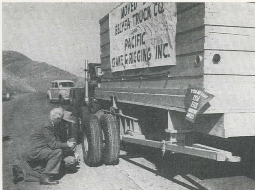
ENGINEERS INSPECT installation of dolly beneath primary trailer. Two 4-wheel dollies constructed in advance and attached by bolts to an I-beam "outrigger" welded to the trailer were estimated to relieve the trailer load by more than 7 tons.
