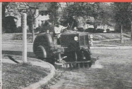
MODEL "40" SWEEPER—Compact, simplified, quick-dumping. May be had with right-hand or left-hand gutter broom, or both. Leaf Broom attachment also available.
