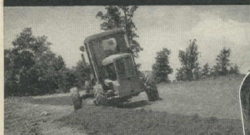
RIDING A LONG SLOPE . . . All-Wheel Steer holds both ends steady.
