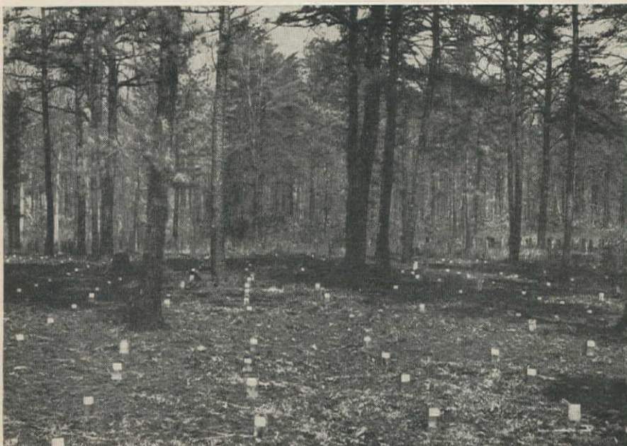
SOIL POISONING experiments by the Department of Agriculture were carried out at the research center at Beltsville, Md. The test area is divided into 10 blocks and untreated wooden stakes are driven in the center of each plot, below. Each fall the stakes are examined and records made by Department entomologists, above.
