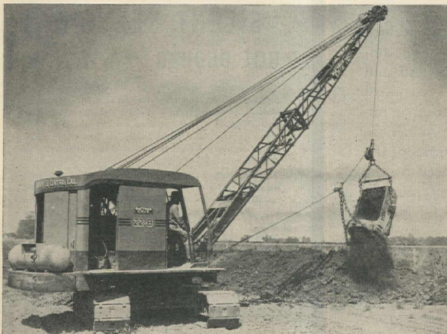
Bucyrus-Erie 22-B Dragline, owned by J. S. McElvany, El Centro, Calif., on drainage excavation in Imperial Valley.
