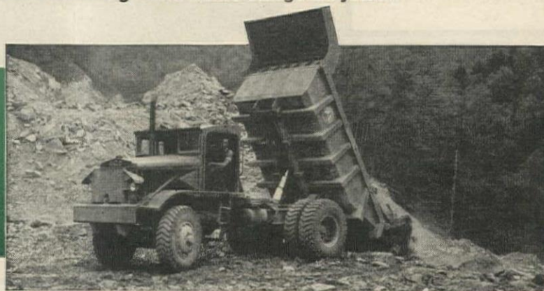
Because of the high dumping angle and distance of the chute from the rear wheels, the load is dumped over the bank.
