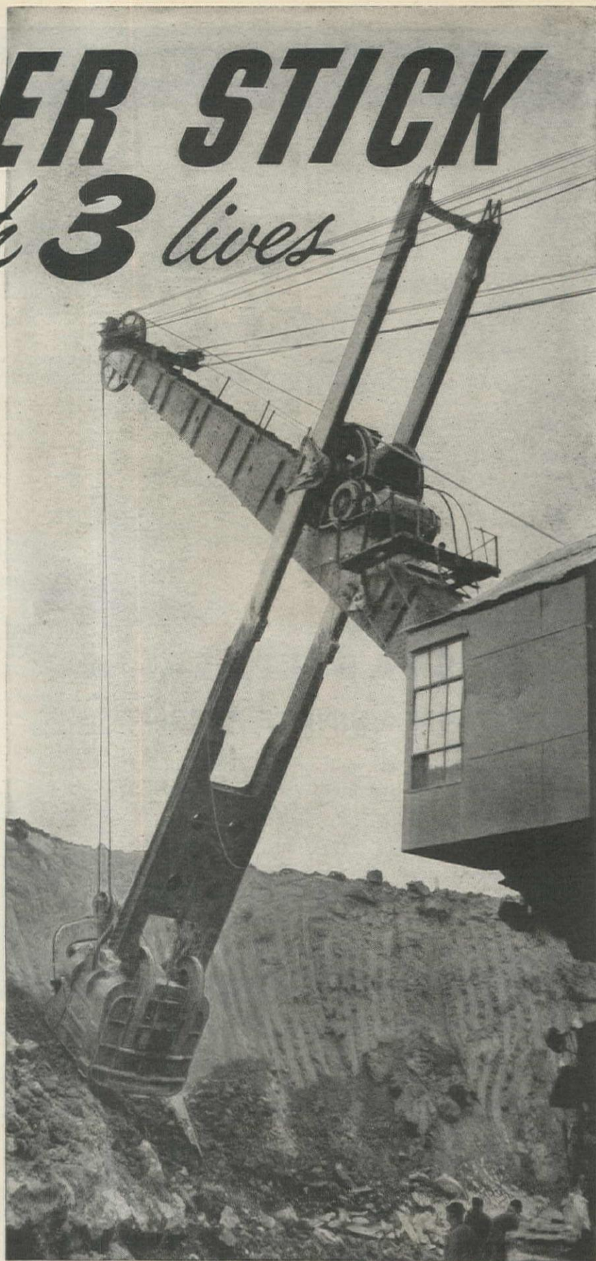
13-cu yd shovel with Mayari R dipper stick. This stick has been in operation for more than 18 months and has required no repairs.
