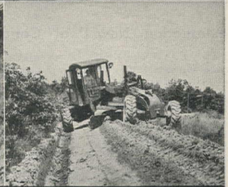
HEAVY GRADING. Controlled Traction moves the windrow up the slope, farther and faster.
