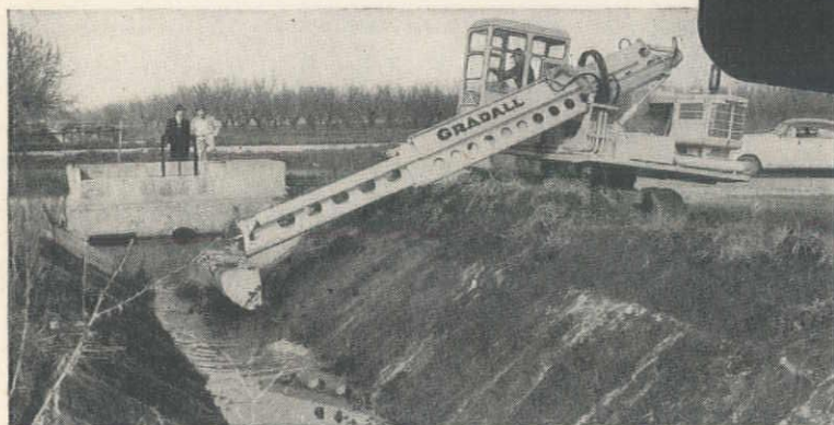
Gradall's fast, agile "Arm Action" guides the bucket down one side of the ditch, across the bottom and up the other side—clean in one pass!
