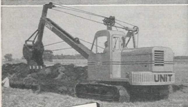
UNIT TRENCHER Crawler-type ditch digger used on large drainage project. Delivers fast, profitable payloads. Quickly convertible.
