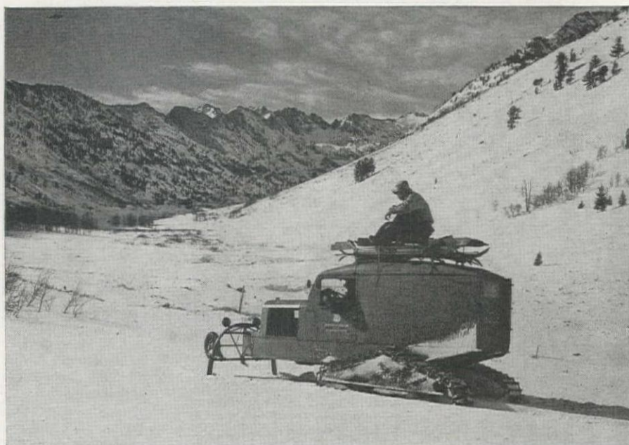
SNOW SURVEYING is now carried out by many agencies using modern over-snow machines instead of the laborious hiking on snow shoes or skis. The machines make possible more extensive surveys in remote watersheds than was possible in early years.
