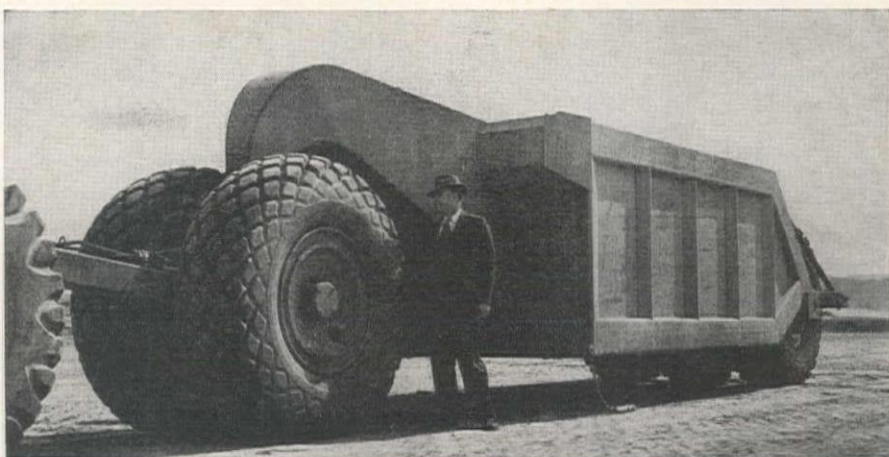
RUBBER TIERED roller purchased especially for compaction of embankment at San Francisco Airport. Its five tires support a weight of 60,000 lb. It was specially built for this work by Southwest Welding & Manufacturing Co. The editor of Western Construction News is dwarfed by the huge machine.
