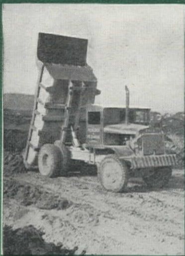
Tapered chute construction and high dumping angle mean quick, clean shedding of the load — an important advantage of Rear-Dump Euclids.
