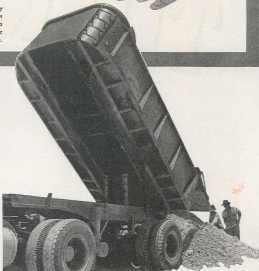
Part of the fleet of Hercules Huskies operated by the R. B. Tyler Company on a road construction project near Miami, Florida. Working 24 hours a day, these semi-trailer dump bodies carry 12 cubic yards per trip over a 44-mile round trip route.
