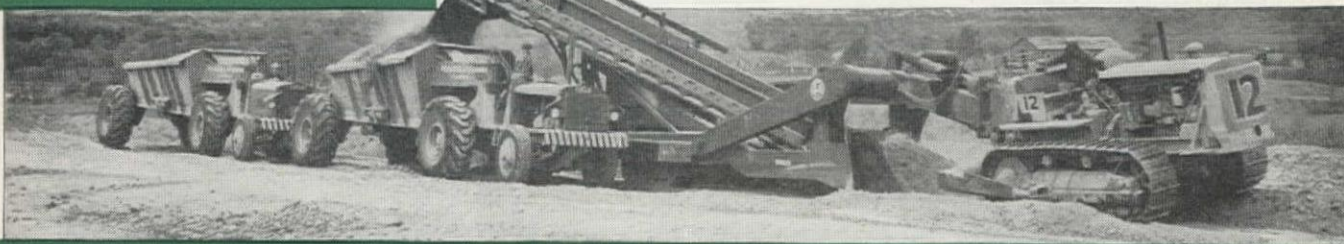
Tapered chute construction and high dumping angle mean quick, clean shedding of the load — an important advantage of Rear-Dump Euclids.
