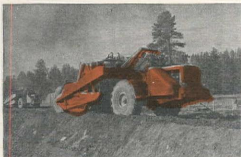
WOOLDRIDGE TERRA-COBRA employ the same Bowl features as Wooldridge "Terra-Clipper" tractor-drawn Scrapers
