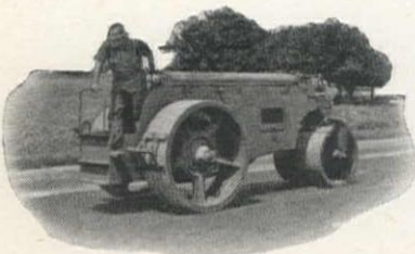
3-WHEELED ROLLERS —Made in sizes ranging from 6 to 12 tons. Gasoline or diesel engines. Hydraulic power steer. Hydraulic scarifier attachment.
