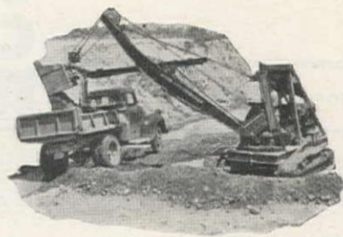
BADGER SHOVEL —Convertible to crane, dragline, piledriver, trench hoe, and skimmer. 3/4-swing design has many operating advantages.
