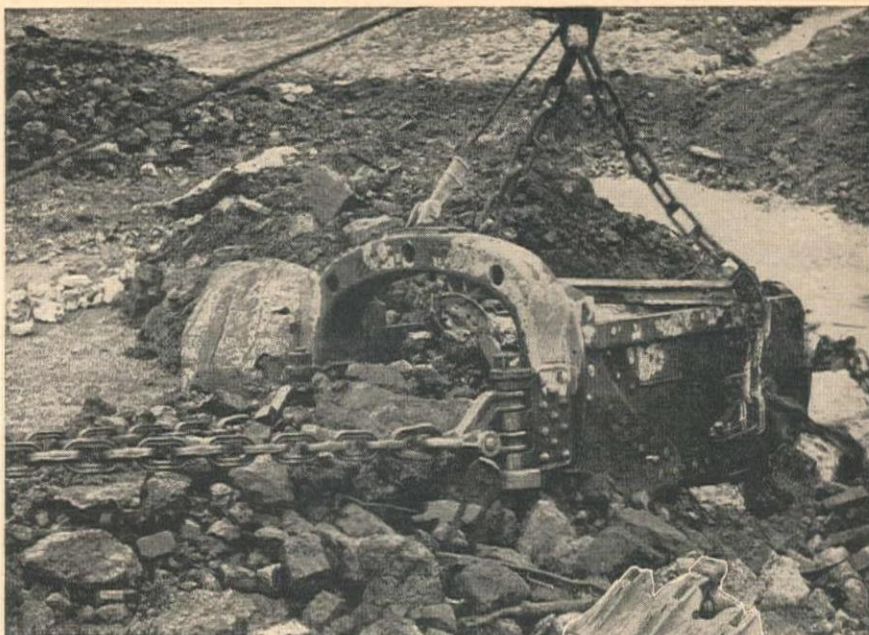
Above: ESCO 1 1/2-yard heavy duty bucket operated on Bucyrus 37, digging steel slag in Republic Steel plant.
