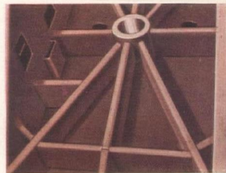
Here you see the interior web-work of strengthening members in the P&H all-welded revolving frame. Sidestands are welded integral. There are no bolted joints — alignment of machinery is permanent.
