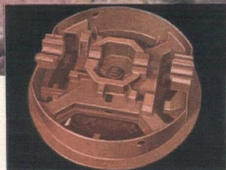
Here's the strongest carbody construction known. Axles are welded integral with turret — and crawler frames with axles. Here's one piece, trouble-free construction.
