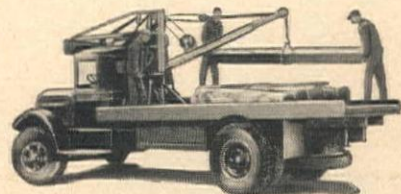
Telescopic boom Crane. Radius 8 to 20 feet.
