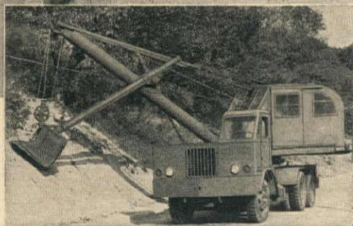
MICHIGAN MODEL TMDT-16 — ½ yd. shovel, 10-ton crane. Equipped with Timken Tandem dual drive axle. Total reduction in low gear 72.88-1. Four Timken-Westinghouse air brakes.
