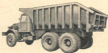
Type X-112 Extra heavy duty Body with automatic downfolding tailgate.
