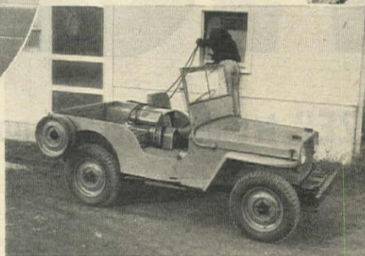
Welding generators (left, center) are available up to 300 amps at 32 volts. Power generators (right) come in 1-, 3-, and 15-kw ratings. Jeep can be supplied with either one or both generators.
