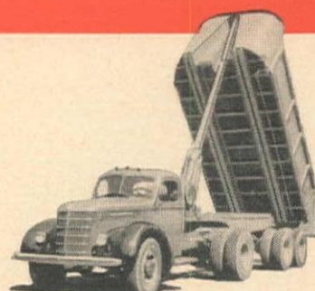
Type W12 Body, front recessed for Model TV83 Hoist. Capacity 15 cu. yds.
