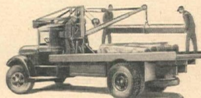
Telescopic boom Crane. Radius 8 to 20 feet.
