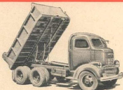
Type W12 Body. Model F4C cam and roller Hoist. Capacity 6 cu. yds.
