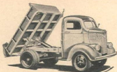
Type C12 Body and Model D6 or D7 Hoist. Dumping angle 55°.
