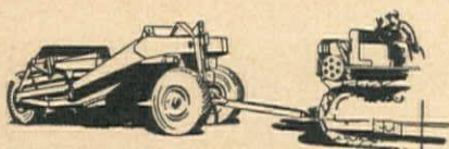
CABLE OPERATED SCRAPERS 6, 8 and 14 yard capacities for use with all makes of crawler tractors
