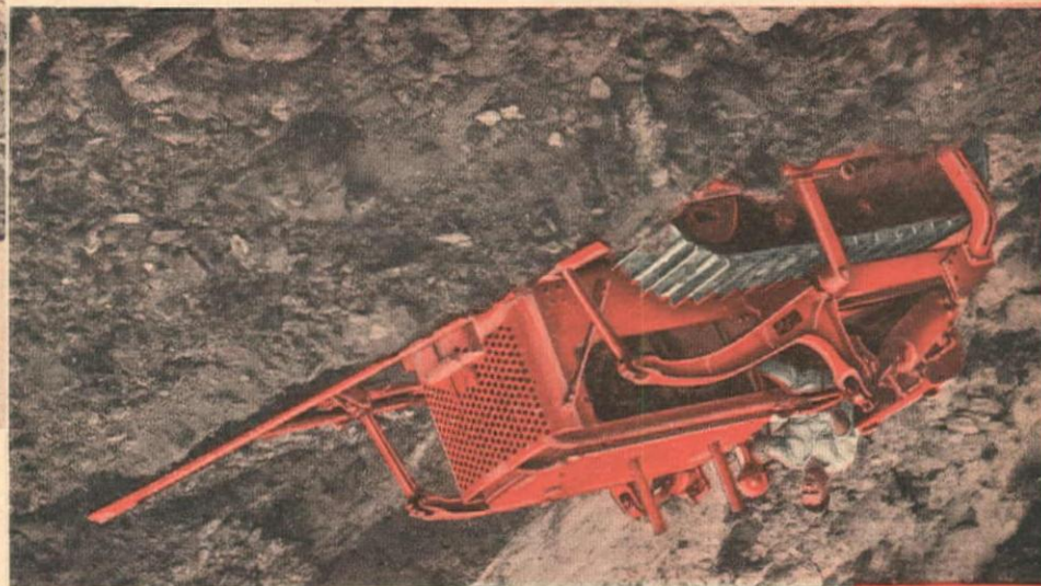
Above: It's a TD-18 Tractor cutting out a roadway on a hillside with a bulldozer blade. Wherever roads are built, International's speed the job, help keep costs down to bedrock.
