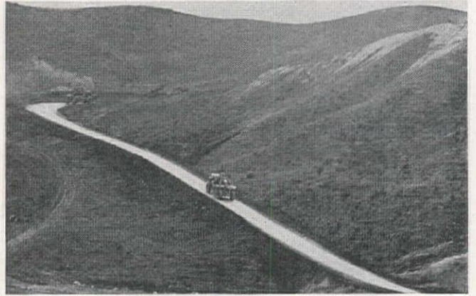
27% Return Grade . . . Tournapulls climb 1000 feet along this 27% grade up the mountain, making it easily in 2nd gear.
