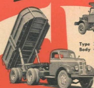
Type Q12 Body with Model T440 dual telescopic Hoist. Capacity 16 cu. yds.
