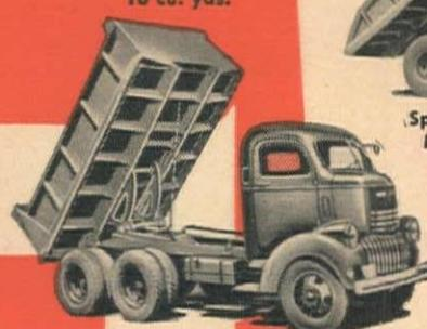
Type W12 Body—Model F4C cam and roller Hoist. Capacity 6 cu. yds.
