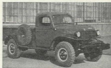
22 $\frac{1}{2}$  in. high. Wheelbase is 126 in. and maximum payload is 3,000 lbs. A dual power take-off is available to deliver 536 rpm. at the tail shaft to operate auxiliary machinery. The power take-off also operates a front-mounted power winch of 7,500 lb. capacity.
