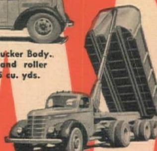
Type W12 Body, front recessed for Model TV83 Hoist. Capacity 15 cu. yds.
