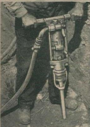
CP Sinker Drills are fully cushioned for low upkeep; valve operated, they maintain their drilling speed despite wear. CP makes a sinker drill for every contracting need, from the light 28-pound CP-22 to 119-pound heavy duty CP-60.
