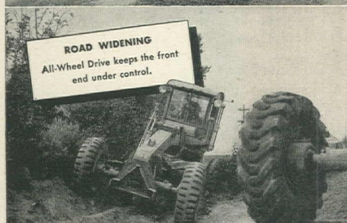
—no Motor Grader without All-Wheel Drive and All-Wheel Steer will be able to match the all-around performance of the "99-M" Power Grader.
