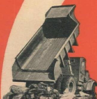
Rock excavating Body with downfolding gate.
