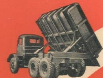
One way side dump Body with dual telescopic Hoist. Automatic downfold side.
