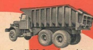
Type X-112 Extra heavy duty Body with automatic downfold tailgate.
