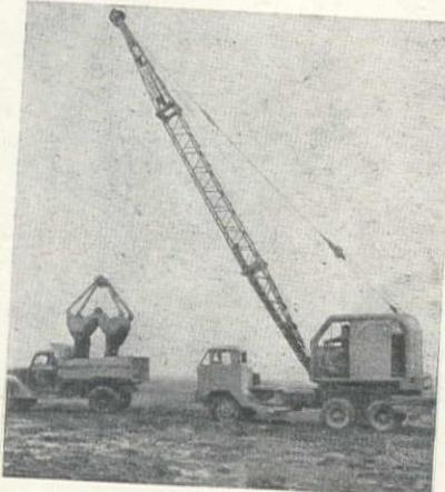
speed when traveling overland or through congested areas. At the job, truck functions are taken over by the crane operator through the "Tu-Control" mechanism. He can move the truck forward, back or around turns with the truck engine shut off, thus assuring precise control over the truck in relation to the load on the boom.
