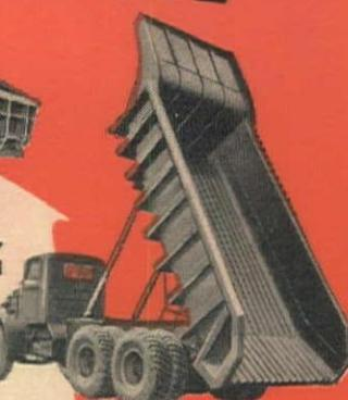
Type X-112 Extra heavy duty Body, scoop end, with Model T-4440 Hoist. Capacity 19 cu. yds.
