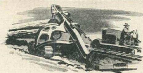
Logging machinery moves dead-weight logs with wire rope providing the sinews. Preformed wire rope gets top billing because it handles easier, resists kinking and stands the gaff.
