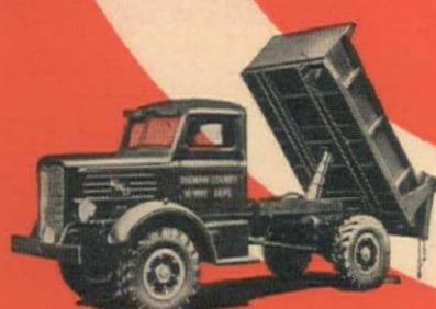
Type W12 Body and single telescopic Hoist. Double acting tail-gate Capacity 4 cu. yds.
