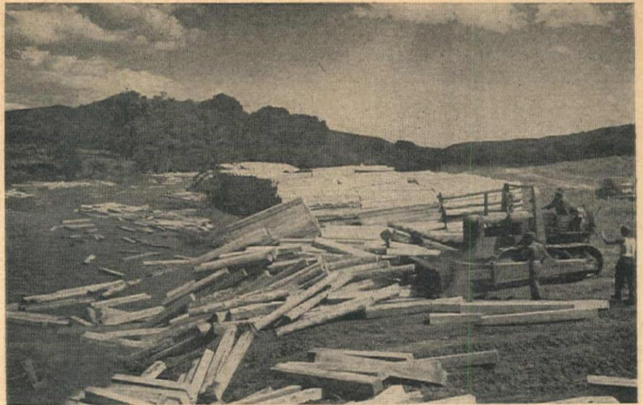
BULLDOZER FOUND EFFECTIVE IN MOVING RAILROAD TIES TO MARKET
