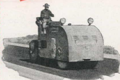
TANDEM ROLLERS —Made in 2 sizes—5 to 8-Ton and 8 to 10½-Ton. The variable weight feature enables one machine to handle a wide variety of jobs.
