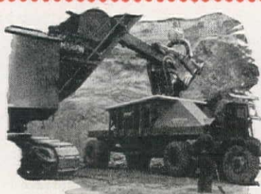
TRAIL CARS —Hopper-bottom and side-dump types. Designed for heavy duty haulage behind powerful truck-tractors, in open pit mines, quarries, etc.
