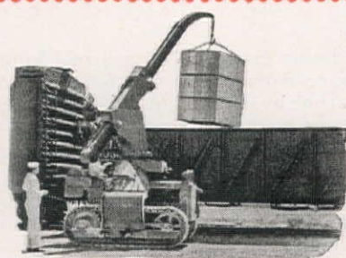
HYDRAULIC CRANE —Retractable-extensible boom provides ability to lift and carry maximum load under such handicaps as low doors and ceilings, inside box cars, etc.
