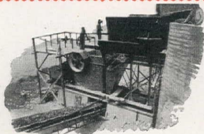
CRUSHING EQUIPMENT —Roller bearing jaw crushers and roll crushers in a wide variety of sizes. Portable and semi-portable crushing and screening plants for all purposes.
