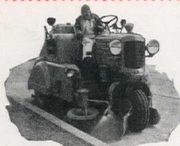
PATROL SWEEPER —Compact, simplified, quick-dumping. Rear broom throws dirt directly into hopper. May be had with Leaf Broom attachment.
