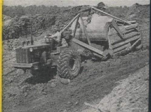
Giant tires of Tournapulls (above) and Tournatrailers (below) take beating of rough rocky jobs with less maintenance than crawler tracks or small truck tires.
