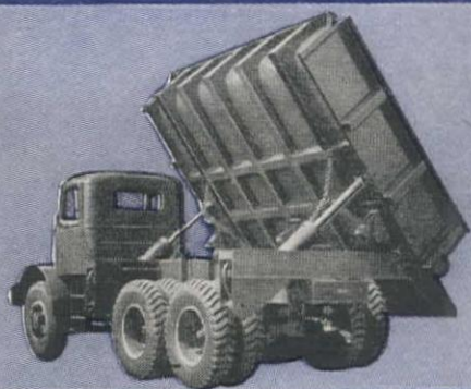
One-way side dump body with dual hydraulic hoist. Automatic downfolding side.
