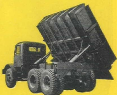
One-way Side Dump, Dual Hydraulic Hoist. Automatic downfold side.
