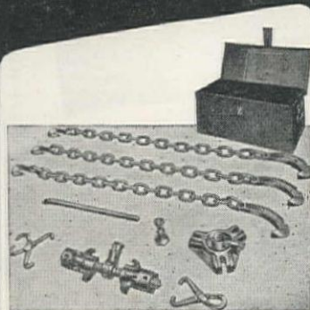
No. 610 Util-A-Tool. 10-ton capacity. Pushes apart or pulls in 4 3/4" each grip. Weight 74 lbs. in metal box.
