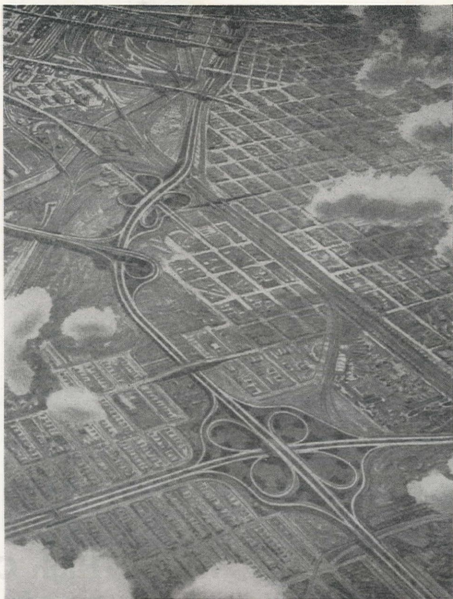
BIRD'S EYE VIEW of the Valley Freeway proposed for Denver, showing various types of connections with cross highways. The view is toward the south. In foreground is the cloverleaf system at 46th Ave., next is 44th Ave. grade separation, the connection to Broadway and the Fox St. interconnection. Freeway then passes over railway and under 20th St. Next are 18th St. ramp system, two viaducts and Speer Blvd. cloverleaf.
