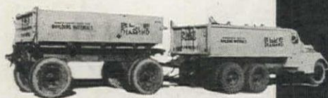
This roll-in type dump Trailer operated by Blue Diamond, Los Angeles, adds many tons to the truck's capacity.
