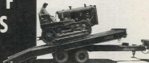
A 10-ton Fruehauf Tilt-deck Trailer, operated by the Emergency Rubber Project of the U.S. Dept. of Agriculture.
