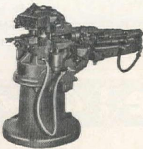
Four sizes of drill steel sharpeners permit the right selection for any job of shanking or threading, etc.
