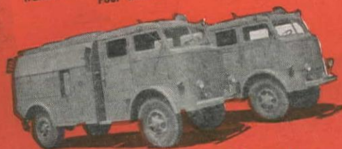
Utility Line Construction and Maintenance trucks by FWD with 5 and 7 man cabs, special power-take-offs and line bodies. Powered with 115 h.p. engine on 144" wheelbase with four-wheel drive, 5 speed transmission, 144" wheelbase and 9:00x20 tires.
