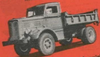
"U" series FWD's with gross vehicle weight capacities of 22,000 to 28,000 lbs. Powered with 125 h.p. gasoline engines, 5 speed transmission, 11:00x20 tires, wheelbase 150". Four wheel drive.
