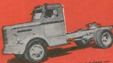
FWD's four-wheel drive Road Maintainer — built for underbody scraper use with extra heavy frame and other features that make it the ideal unit for street and road maintenance. Engine 115 h.p. — 5 speed transmission — 8:25x20 dual tires.
