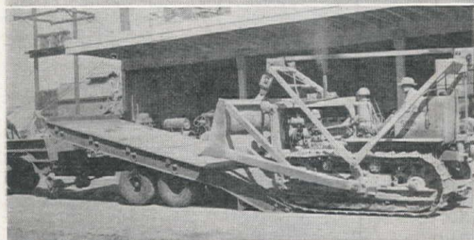
You can hardly see the Trailer under this huge 66-ton superstructure assembly at Consolidated's Wilmington Shipyard. Yet the load is only a "light haul" for this Fruehauf Trailer, which was built to carry an emergency load of 125 tons.
