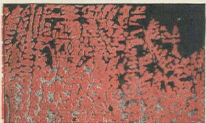
Top Photo: A photomicrographic cross-section shows the lead component of a new copper-lead bearing in light grey. The copper is shown as red. Note the even distribution throughout.
