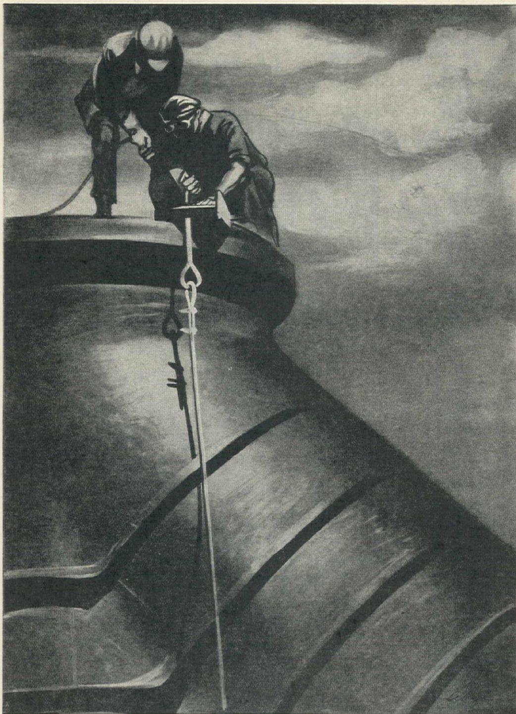
72-inch flanged Y-Branch weighing 17 tons being secured to special underslung car for rail shipment to a War Project. Drawn by Rico Lebrun for U. S. Pipe & Foundry Co.
