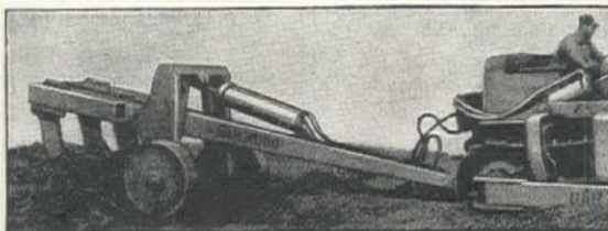
2F Rippers rip compacted earth, shale, rock, roots, old pavements, old roads.
