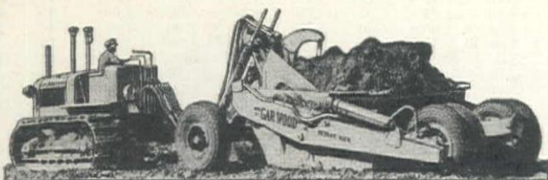
2A 4-wheel hydraulically operated Scrapers for earth moving, specifically constructed for fast digging, easy loading, accurate spreading.
