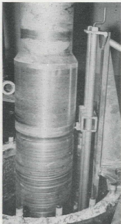
THE VERTICAL lathe has been set in place and the cutting tool in the movable tool holder carriage is taking the first cut.
