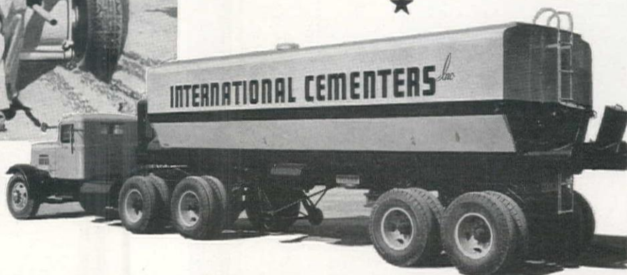
The bulk cement Trailer first hauls the cement, then spreads it. Upon arrival at the job a spreader is attached to the rear end, into which the cement is moved by two screw conveyors in the bottom of the Trailer hopper.
