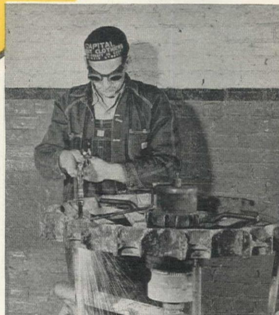
Cutting off a worn sprocket rim with acetylene torch
