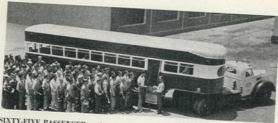
SIXTY-FIVE PASSENGER trailer-bus, manufactured by Fruehauf Trailer Co., of Los Angeles, Calif., is used to transport shipyard workers to and from their work at Marin shipyard of Bechtel Co., near San Francisco.
