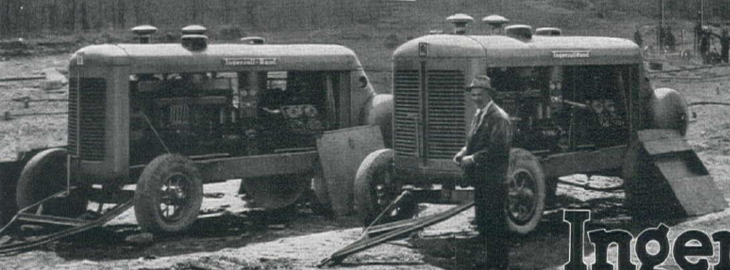
500-CFM MOBIL-AIR COMPRESSORS EACH OPERATING TWO WAGON DRILLS
