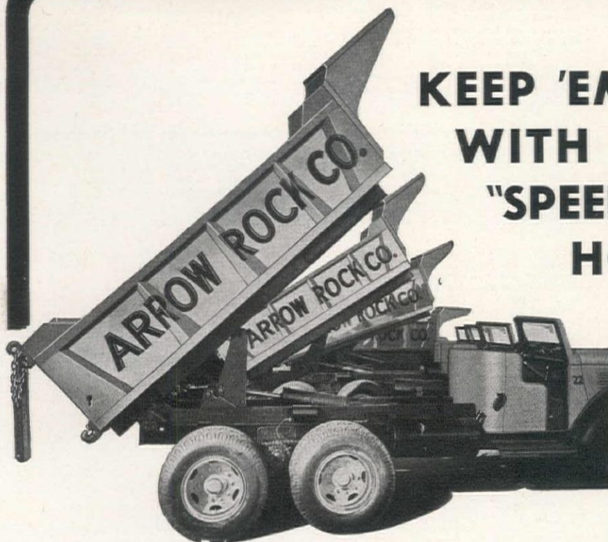
8X SPEEDRAULIC Hoists and 6 cubic yard dump bodies used for heavy excavation work.
