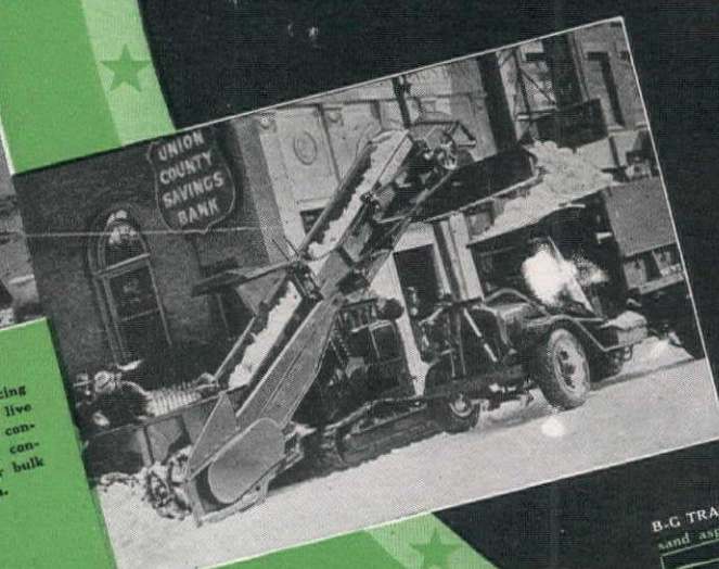
B-G "GOOSENECK" COAL LOADER . One of many being used for handling coal and coke for heating hangars and airport offices both in the United States and Canada.
