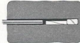
Another cartridge goes in—Compaction takes place inside the wrapper.
