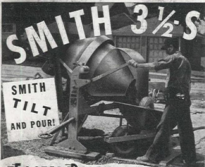
You merely tilt the Smith drum thru a short 40° arc and let gravity pour out the entire batch . . . the quickest, most practical and most convenient method of discharge . . . like emptying a pail. Returning to charge position, the drum again moves through a short 40° arc. More time saved! Contrast this quick, short tilt with the long, time-consuming 180° tilt of all other tilting mixers. Seconds saved with every batch means a BIG saving over a period of years.
