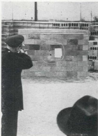
stop .30 caliber military rifle and machine gun fire at distances as short as 10 ft. Blocks are lightweight, made with blast furnace slag. Especially useful in protecting transformers, utility stations, and vulnerable industrial equipment.
