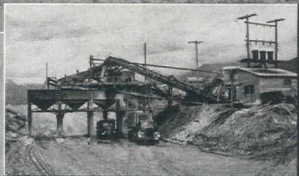
(A) Over-all picture of the installation, showing Pioneer tandem screens mounted over loading bins.
