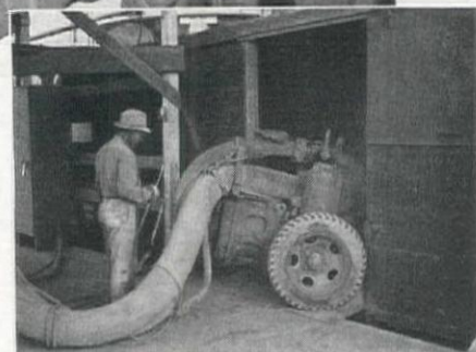
Fuller-Kinyon Remote-Control Unloader unloading cement from box car.
