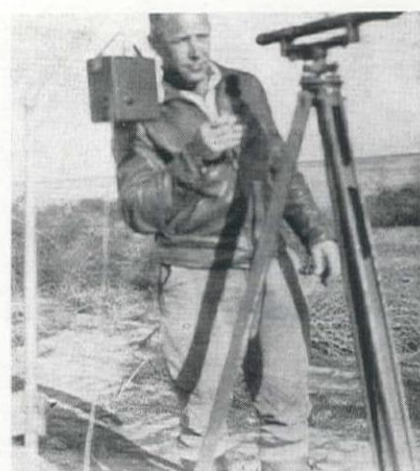
MICROPHONE and amplifying system in a small box are suspended from a light standard near the instrument to receive rod readings called by levelman.
