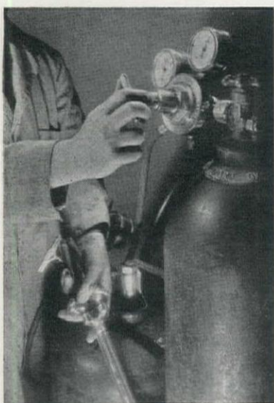
8—Adjust oxygen regulator.....
