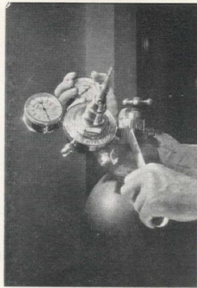
3—Attach oxygen regulator.....
