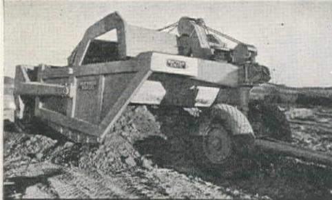
Side plates are extended well ahead of the cutting edge to eliminate side spilling of dirt while spreading or loading.
