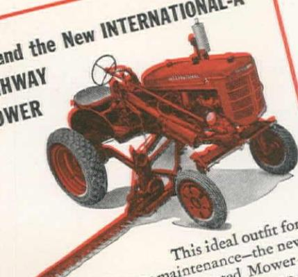
This ideal outfit for highway maintenance—the new International-A Side-Mounted Mower—cuts a 5-ft. swath at mowing speeds up to 6 m.p.h. Cuts at any angle from 90° above horizontal to 45° below horizontal. Pneumatic power-lift controls angle of cutter bar. Enclosed, heat-treated gears run in oil bath. Electric starting and lighting.
