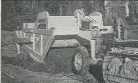
The dirt rolls easily out of the bowl and underneath the scraper; no power wasted bulldozing it under.
