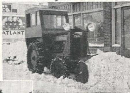
The four basic sizes of Case industrial tractors are furnished with a wide choice of wheel and tire equipment, affording an unbroken range of weights from 2400 to more than 11,000 pounds. Thus they can be closely matched to maximum traction requirements as well as to power and speed range. All are available with mounted equipment designed especially for them by foremost manufacturers.
