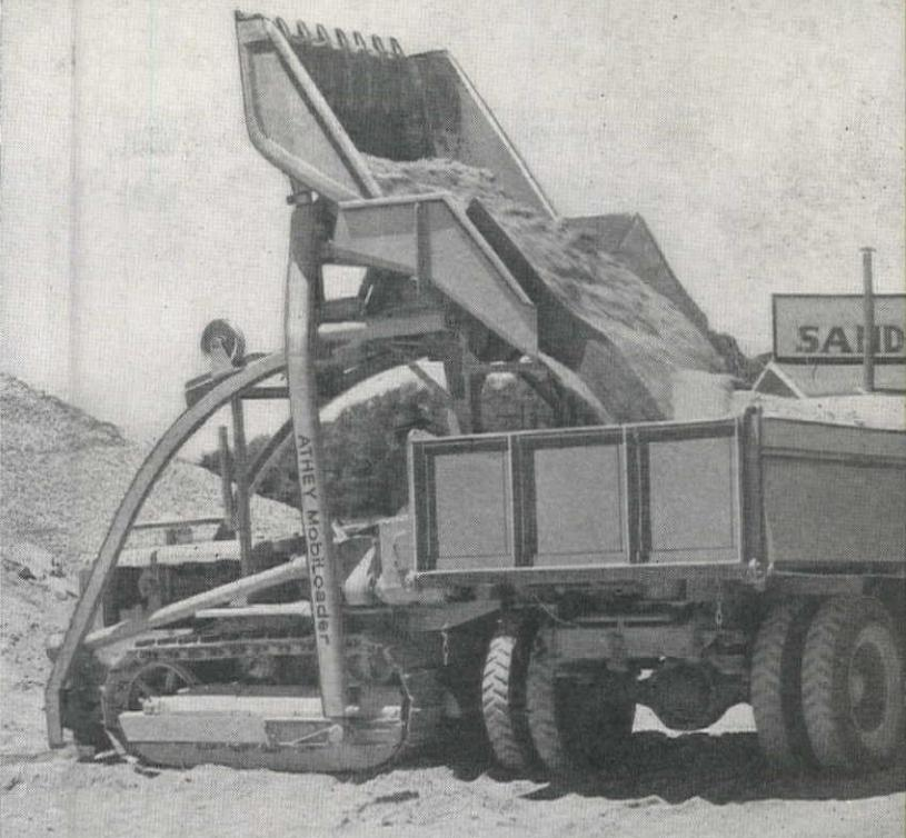
*Stock pile loading—20-foot haul from pile to truck—at 120 cubic yards per hour.*
