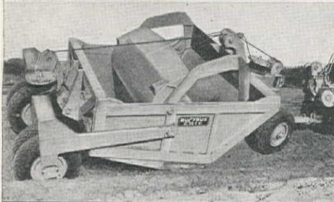
Load can be dumped and spread on side slopes because of accurate control, wide wheel spread, and low center of gravity.
