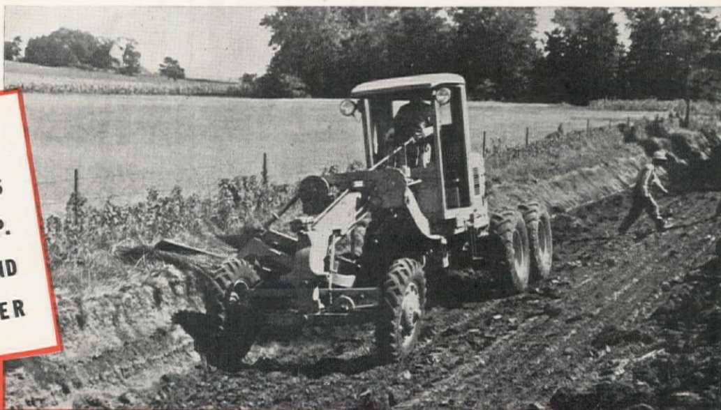
● Adams Heavy-Duty Motor Grader No. 511 with 68½ h.p. Diesel engine; same machine available with 66½ h.p. gasoline engine.
