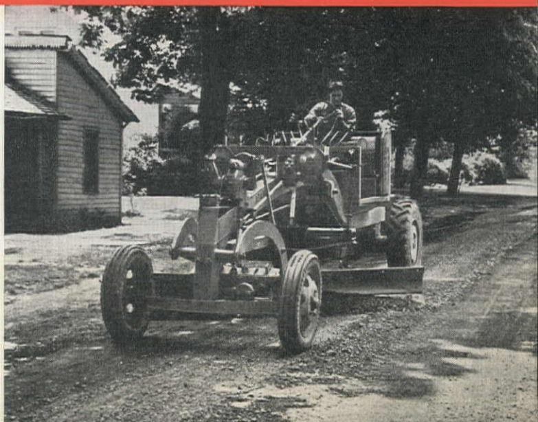
● Motor Grader No. 201 with 31 h.p. gasoline engine—a low-price machine for surface maintenance and light ditch and bank work . . . All Adams motor graders are of the high-lift, bank-cutting type.
