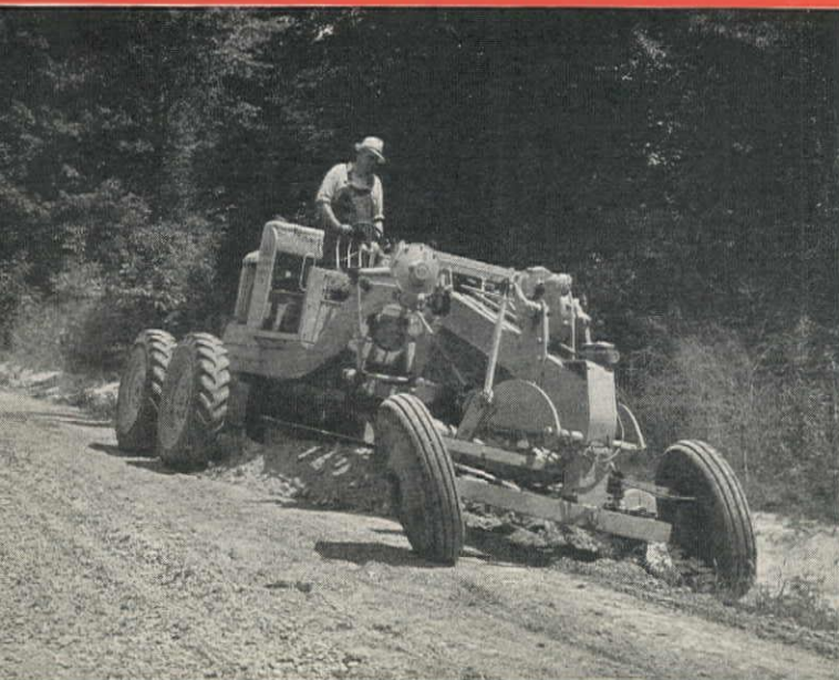
● Adams Motor Grader No. 311 with 50 h.p. Diesel engine; same machine available with 45 h.p. gasoline engine. Same type machine also available with 68½ h.p. Diesel engine—a high-speed, heavy-duty machine.
