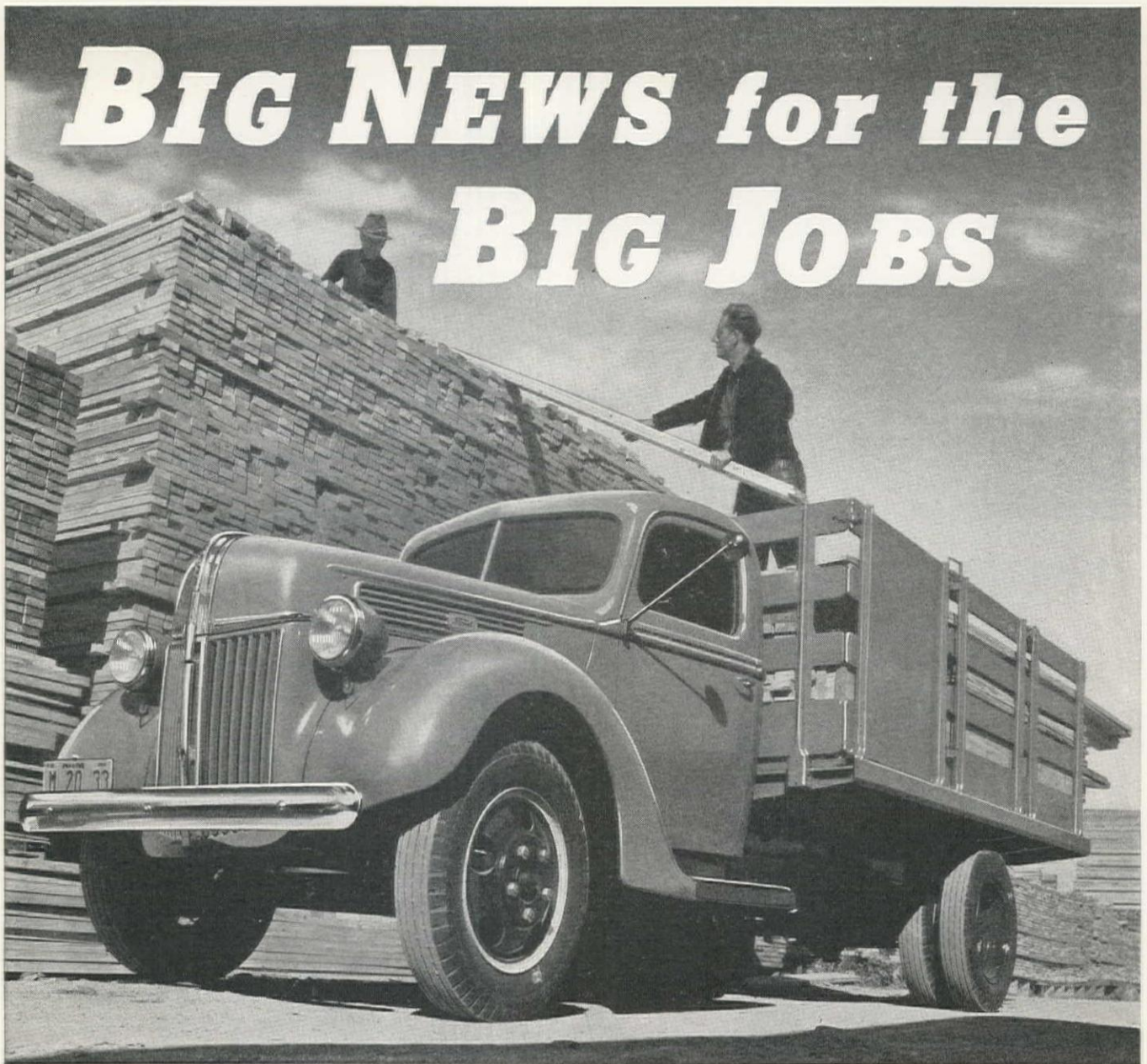
158" wheelbase Ford Truck powered by an 85 or 95 H.P. engine is ideally suited to meet 95% of all general hauling requirements.
