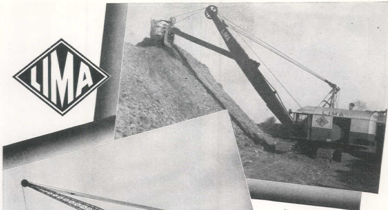
Above—LIMA Type 1201 Shovel owned by Peterson Coal Co., Beloit, Ohio. This machine is equipped with a 42' boom, 32' dipper handle and 2½ yard dipper.
