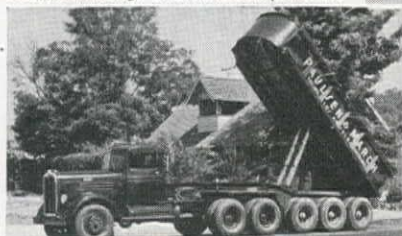
68,000 LB. GROSS WEIGHT, 18 TO 19 TON PAYLOAD. Heil Telescopic Hoist with 15 to 17 cu. yd. Dump Body, 21 ft. long. Three Axle Dumping Trailer.
