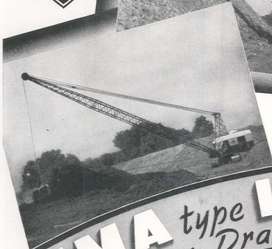
Left—LIMA Type 1201 Dragline, owned by L. E. Harris, Dundee, Mississippi. This machine is equipped with a 90' boom and a 3 yard bucket.
