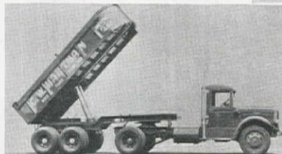
52,000 AND 60,000 LB. GROSS WEIGHT, 15 TO 17 TON PAYLOAD. Heil Telescopic Hoist with 12 to 14 cu. yd. Dump Body, 18 ft. long. Dual Axle Dump Trailer.
