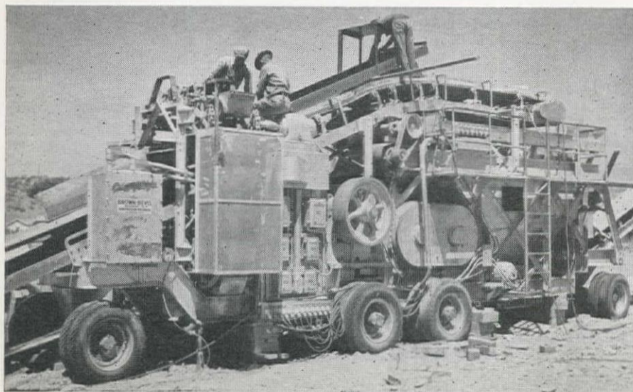
ASSEMBLING the portable plant which travels as two trailer units, separated between the center sets of tires—Complete push-button controls are available for the operator.
