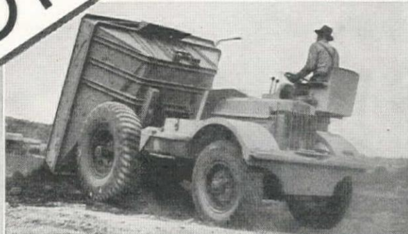
The load is instantaneously dumped by force of gravity, without time-losing mechanical complications.
