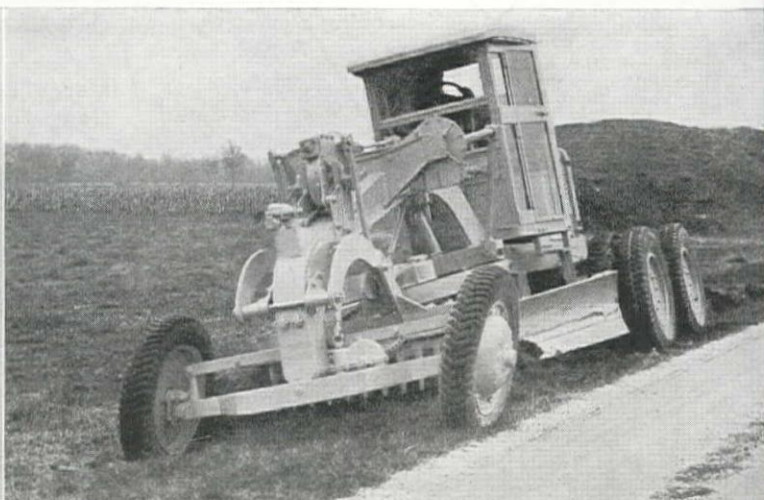
A long front axle with adjustable leaning wheel is available as optional equipment on either machine.
