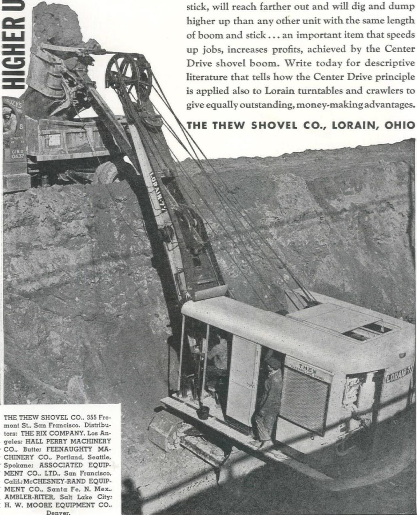
A Lorain-77, with 22 ft. boom and 16 ft. dipper stick, will reach farther out and will dig and dump higher up than any other unit with the same length of boom and stick... an important item that speeds up jobs, increases profits, achieved by the Center Drive shovel boom. Write today for descriptive literature that tells how the Center Drive principle is applied also to Lorain turntables and crawlers to give equally outstanding, money-making advantages.
