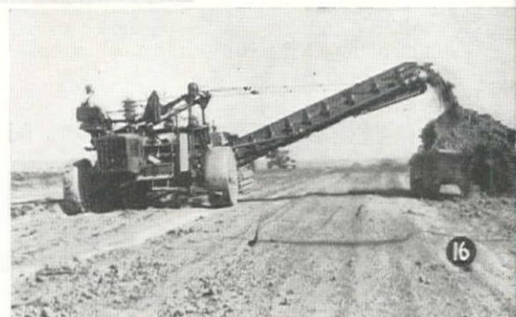
15—On Bonneville dam excavation work this 30-yd. Le Tourneau buggy indicates the action of the oscillating axles in distributing the load on the sixteen 13.5 x 20 tires.
