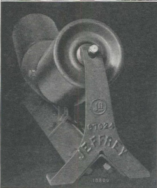
Close-up of Jeffrey Reliance Belt Idler used on the Grand Coulee job. Furnished with 4", 5" or 6" dia. rolls, for belt widths up to 60". Also Jeffrey Hercules Heavy Duty Belt Idlers.
