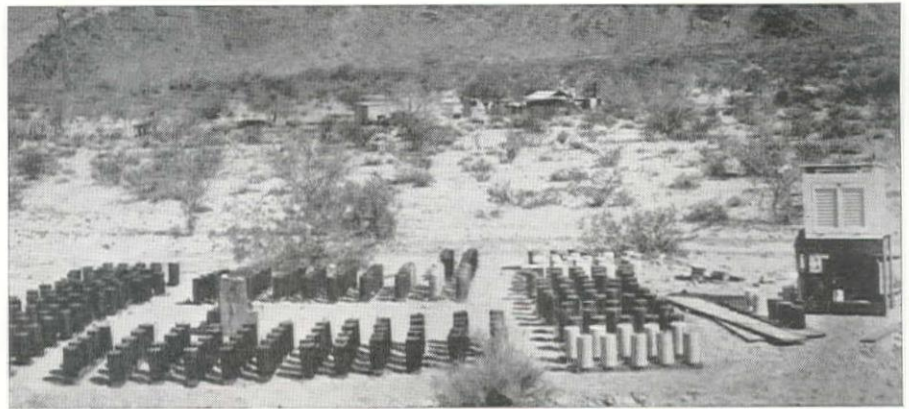
Fig. 1—Exposing the coated 6x12-in. concrete cylinders to typical desert conditions. In the white slatted box is Weather Bureau equipment for observing temperature and humidity. Scales used to obtain frequent weights of the specimens to determine the moisture lost from the concrete were kept under the box in the center.
