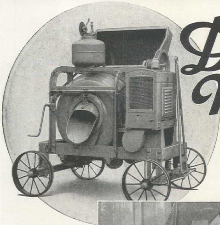
The Koehring Automatic Skip-Flow Shaker, shakes the skip perpendicularly, without strains to the mixer. The aggregate moves along the natural flow-line of the skip.
